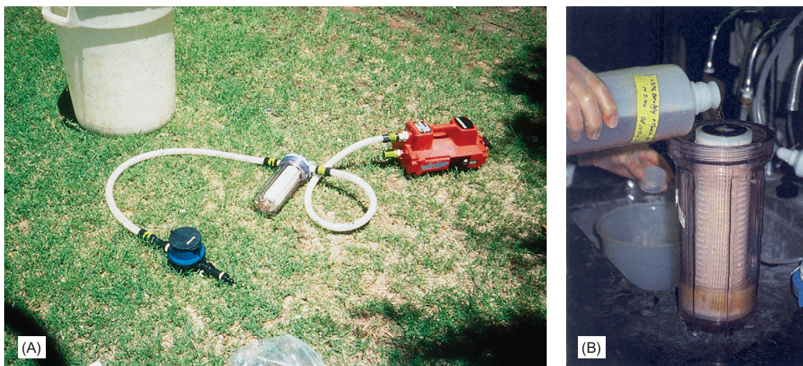
FIGURE 8.7 (A) Field VIRADEL system for concentrating viruses from water. (B) Elution of virus from filter with beef extract.
