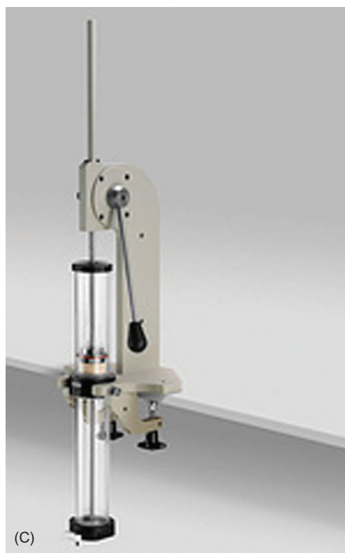
FIGURE 8.9 Filters used for Giardia and Cryptosporidium concentration from water. (A) Environcheck ® Pleated Cartridge filter; (B) Filta-max ® foam filter; (C) plunger system for elution of Filta-max filter. (A) Photo courtesy Pall Filter, Ann Arbor, MI; (C) Photo courtesy IDEXX, Westbrook, ME).
