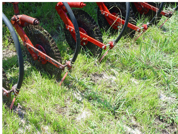
FIGURE 26.4 Liquid manure injection: coulters cut a path in the pasture with injectors applying swine liquid manure effluent below the surface in a furrow. Photo courtesy J.P. Brooks.
