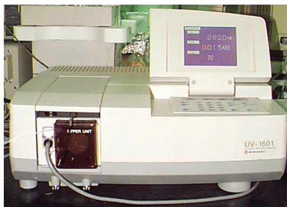
FIGURE 11.1 UV spectrophotometer. Photo courtesy R.M. Maier.
