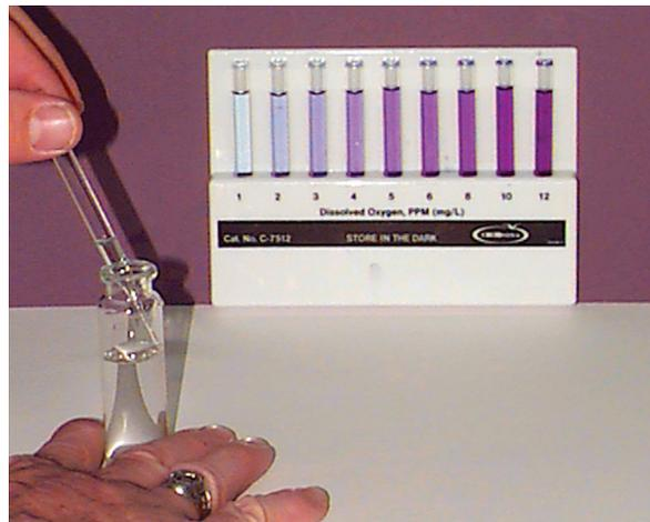
FIGURE 11.9 Oxygen measurement using a Chemets Kit. Photo courtesy R.M. Maier.
