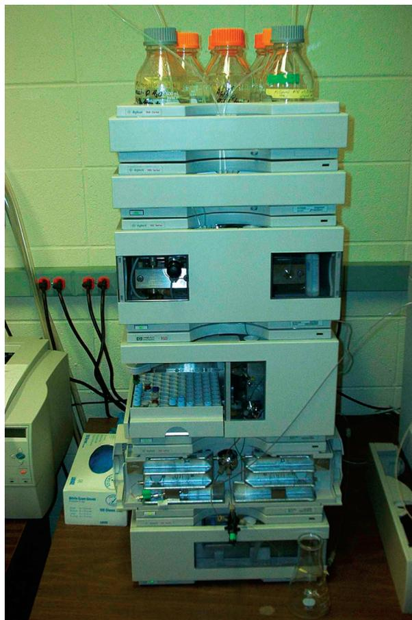
FIGURE 11.4 High performance liquid chromatograph. Photo courtesy T.R. Sandrin.
