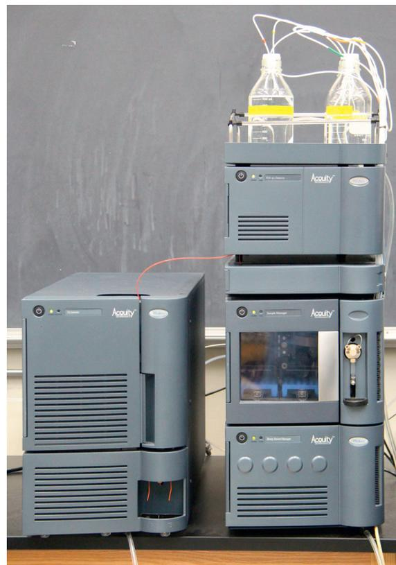
**FIGURE 11.6** Ultra performance liquid chromatograph-mass spectrometer (UPLC-MS). Photo courtesy L. Dykes.
